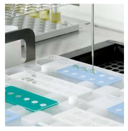
**Caption:** Close up of Fluid RI-1393 preparation being injected onto a blue 10-sample ImmuGlow slide for microscopy analysis, using a Cambridge Life Sciences Ltd model C robotic tray handler.
